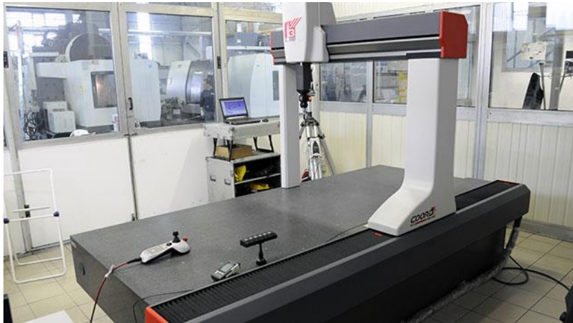
CMM measuring machines COORD 3 HERA SP 24.10.9 2400x1000x900
