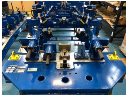
Jigs Pylon A330
